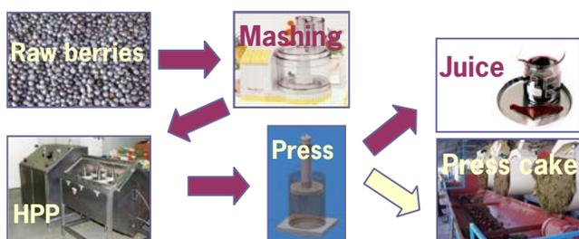
Figure 1. High pressure processing during juice production on laboratory scale.
